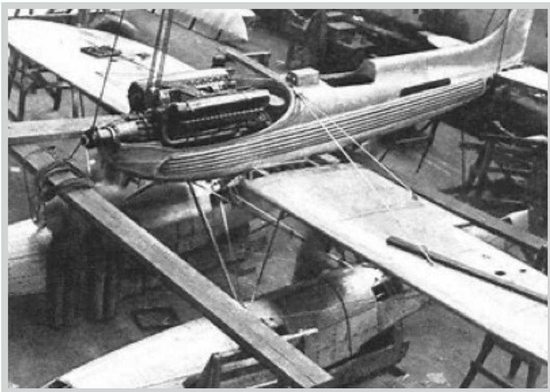
*Supermarine S6B showing the new Rolls-Royce R engine.*
