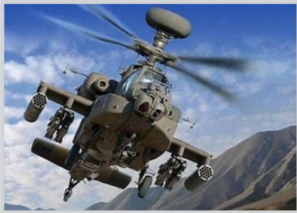
*Boeing AH-64E with Longbow radar to enable 'nap of the earth' flying*
